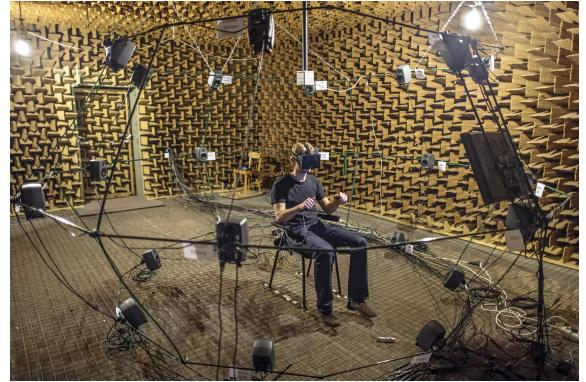
Figure 4: Listening tests were conducted in an anechoic chamber equipped with 24 loudspeakers for spatial reproduction.
